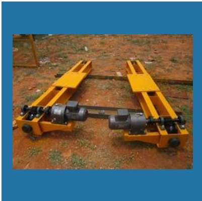
End Carriage Crane
